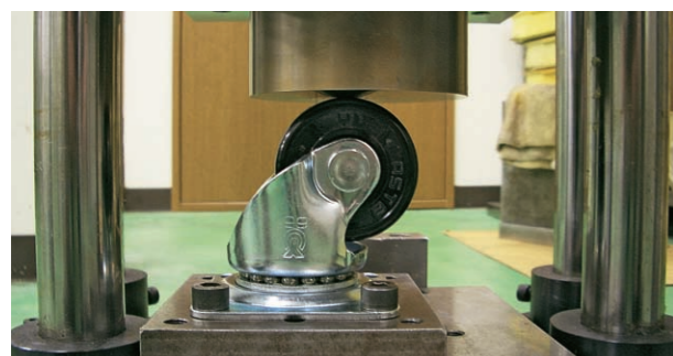
Drop hammer-type impact testing machine
